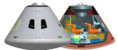
TEACHER RESOURCE 1: Vertical Cross-section of Orion (NASA Concept)
