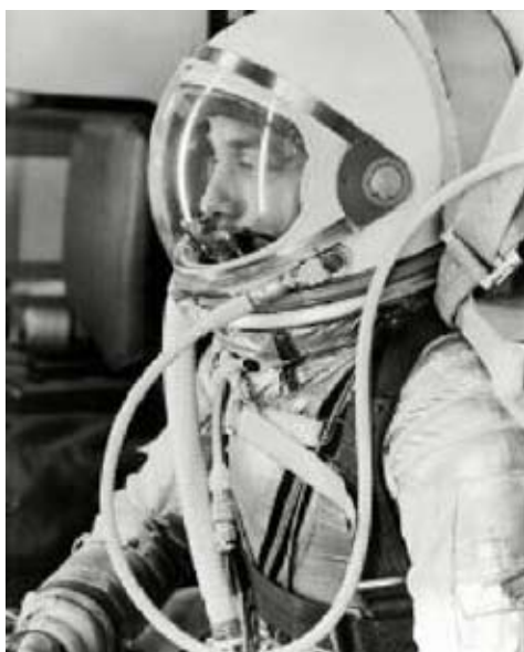
Image: NASA Alan Shepard in Mercury Space Suit showing Hoses for oxygen and cooling
